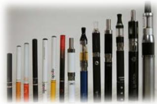
Most e-cigarettes are long plastic tubes (approximately 8 -12 cm) that contain a small reservoir for the oil and a burning chamber that contains a small wick. A button on the tube is pressed and a small battery provides power causing the wick to heat and vaporize the oil. Most basic e-cigarettes can be purchased for \$10 - \$15, while more expensive forms look just like conventional cigarettes and can cost up to \$50.
